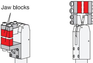
For the fixing and precise positioning of clamping arms and jaw blocks, centering guide bushings GN 870 are also used. The individual data sheets give further information.
