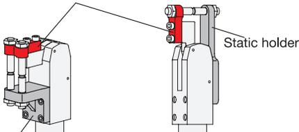
There is an extensive range of accessories available for power clamps, such as tool holders (for clamping arms) thrust bolts and clamping jaws. The sketches shown on the right give some idea.
