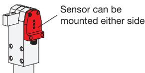
All power clamps can be fitted with proximity switches (inductive sensors) to monitor the end position of the stroke.
