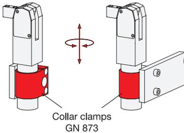
Mounting of the cylinder by a collar clamp increases the numerous ways they can be installed.
