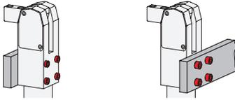
The mounting holes on the main body of the power clamps have been designed to allow installation direct on the internal threaded holes or alternatively with through bolts.
