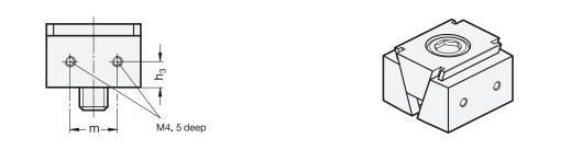
Type **RF** ribbed clamping surfaces
