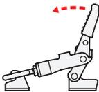
Lift the clamping arm until the latch bolt disengages from the catch.
