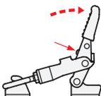
The clamping arm engages in the catch if the release button is pressed for the clamping operation.
