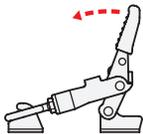
For **clamping operation**, lift the clamping arm until it rests on the catch.
