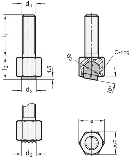
Application example of different clamping pads with O-ring
