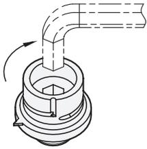
Screw in lower part using an Allen® wrench.
