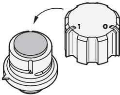
Place upper part on top. The knobs on the upper part and the appropriate recesses in the lower part serve to assemble the unit in the proper and accurate position.
