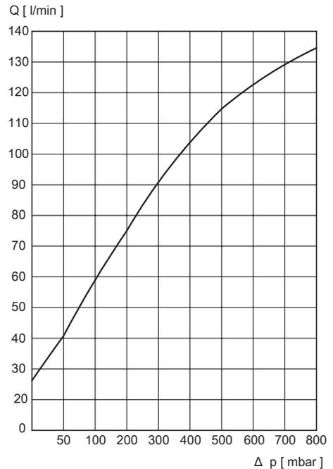
Air flow rate [l/min.] is a factor of the pressure difference [l/min.] between container and ambient air.
