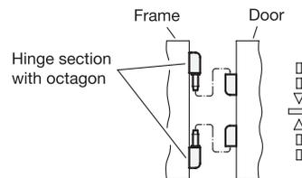
The top hinge section may be mounted to the frame only after the bottom hinge has been hung.
