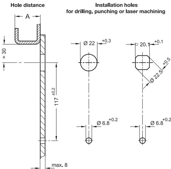
For installation, the door, cover or hatch is fitted with two holes according to one of the two outline drawings.
