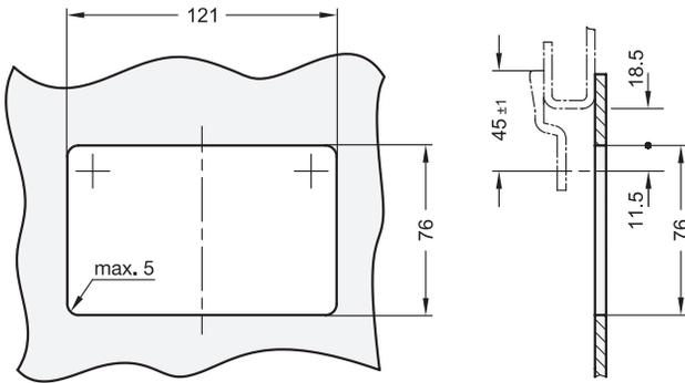
The installation recess in the door, cover or hatch for mounting the latch with gripping tray, must be cut as shown in the outline drawing.
